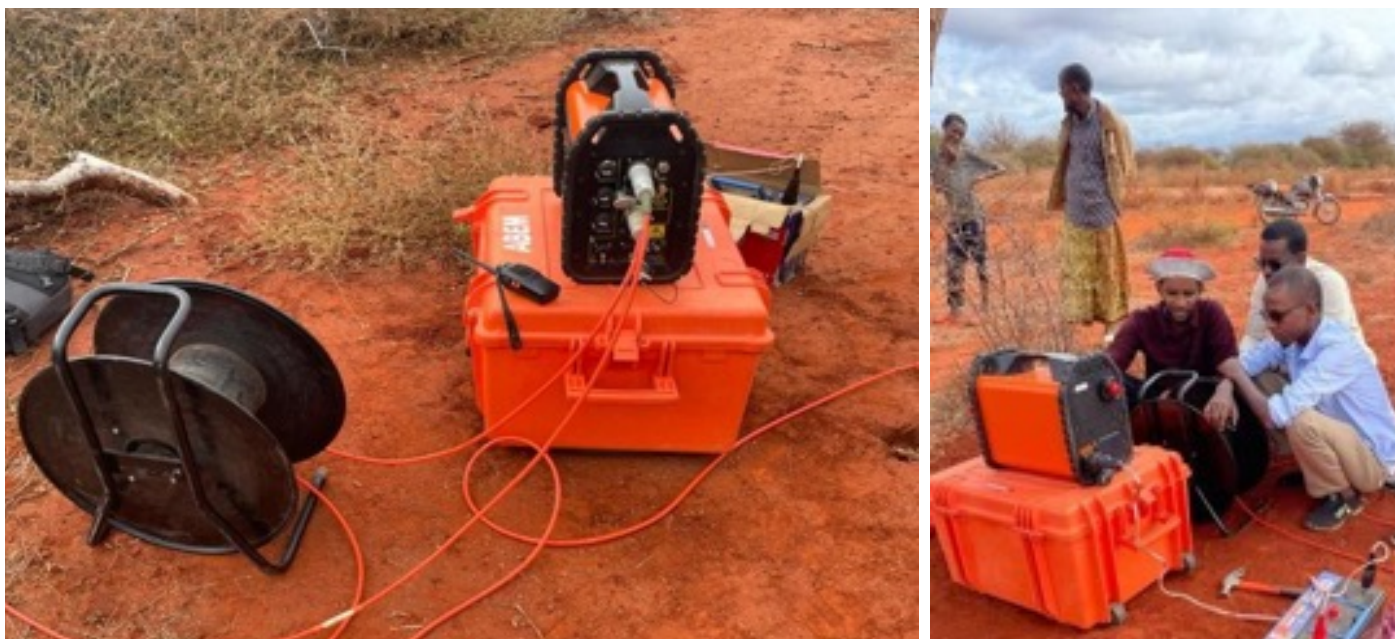
Water Resource team conducting hydro-geological survey in Takaba Town using the ABEM LS2
